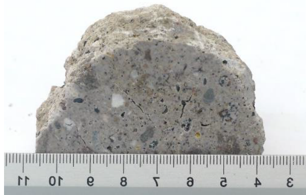
Figure 10: 84% of the material consist of \text{CaCO}_3 . In addition fragments of silicate minerals such as olivin, pyroxene, Al-Ca-fe containing garnets and Mg-Al-Ti containing spinel occur.
