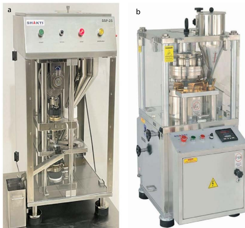
Figure 4: Different types of compression machines used in pharmaceutical development a) Lab model Single Punch Tablet Press and b) Pilot/commercial Scale Single Rotary Tablet Press.
