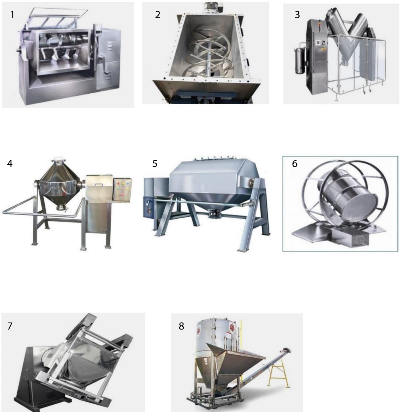
Figure 1: Different types of Pilot/commercial scale model blenders used in pharmaceutical blending unit operation; 1. Mass Blenders; 2. Ribbon Blender; 3. V Cone Blenders; 4. Double Cone Blender; 5. Octagonal Blender; 6. Drum Blender; 7. Bin Blender; 8. Vertical Blender.
