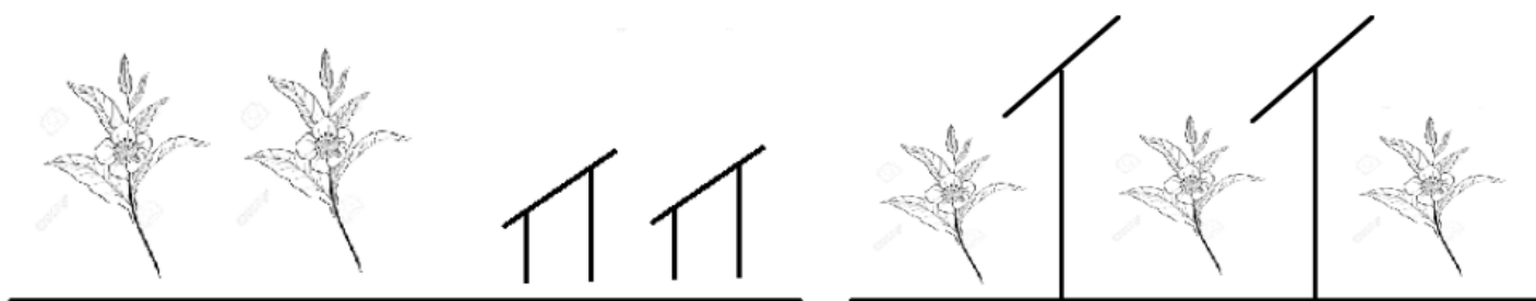
Figure 5: Co-locating SPV and crops on the same owned land in two configurations: (left) separate land with standard-mounted SPV, (right) high-mounted SPV in-between crops.
