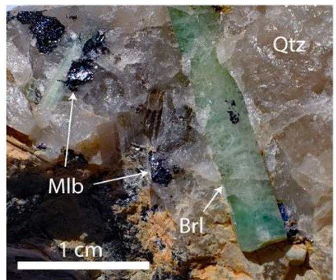
Figure 4: Detail of the studied quartz-beryl sample from the Sauberg mine near Ehrenfriedersdorf: Brl - green beryl, Mlb - molybdenite, Qtz - quartz [33].
