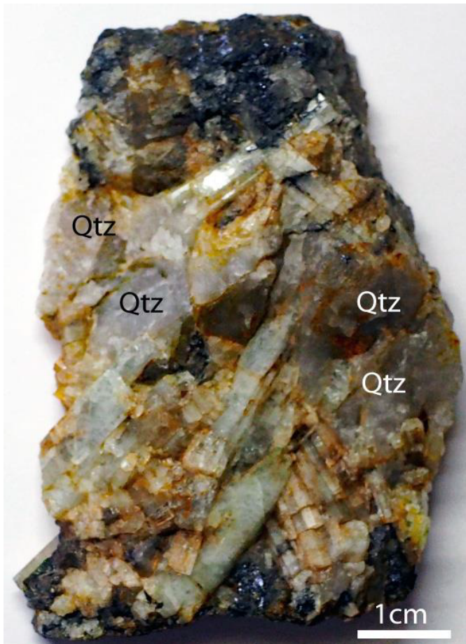
Figure 1: Specimen from a beryl-rich quartz (Qtz) vein from the Sauberg mine near Ehrenfriedersdorf. The sample is from a vertically directed vein - is rotated by 90°. The dark minerals on the roof and the bottom are cassiterite, molybdenite, and other minor ore minerals.
