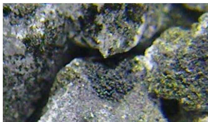
Figure 7: \text{CO}_2 reacts with pyrophoric iron as an oxidizer.
