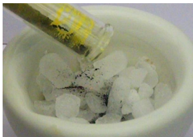
Figure 6: Sprinkling of pyrophoric iron on dry ice.
