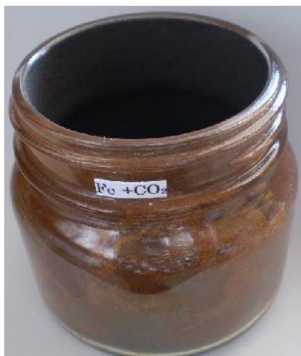
Figure 4: Iron powder with dry ice in a bottle.
