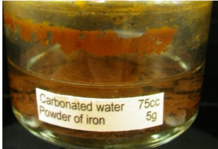
Figure 4: Floating materials were oxidized at a) floating state, and b) precipitate state.
