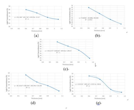
Figure 8: the relationship on the sample for Light Transmissivity vs. Thickness with equation for CF-PVA: (a) Sample-01: CF:PVA of 0.1:30 (0.33%), (b) Sample-02, CF:PVA of 0.2:30 (0.66%), (c) Sample-03, CF:PVA of 0.3:30 (1%), (d) Sample-04, CF:PVA of 0.6:30 (2%), and (e) Sample-05, CF:PVA of 1:30 (3.33%).
