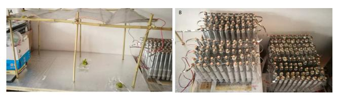
Figure 14: Aluminum-air batteries with K<sub>2</sub>SO<sub>4</sub> electrolyte (a) compose in 200 single aluminum air batteries with 12V and 20 mA for PVA-CF transparent conductive film, (b) To parallel connect 10 single battery and series connect 20 battery groups and all in one.
