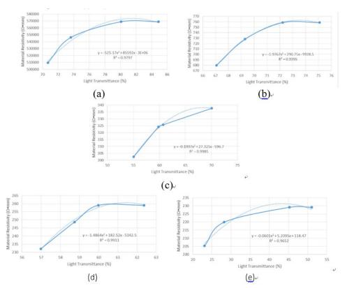
Figure 10: the relationship on the sample for Material Resistivity vs. Light Transmissivity with Equations. (a) Sample-01, CF:PVA of 0.1:30, (b) Sample-02, CF:PVA of 0.2:30, (c) Sample-03, CF:PVA of 0.3:30, (d) Sample-04, CF:PVA of 0.6:30, (e) Sample-05, CF:PVA of 1.0:30. Note: R2 is the percentage of the dependent variable variation that a linear model explains.
