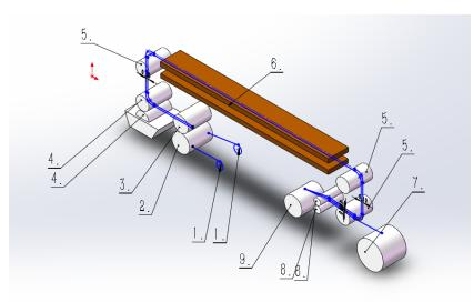
Figure 13: Modified food packaging machine for application of metal copper foil strips and protection laminate. Blue line indicates the feed path of the film. 1: current-carrying, 2: PVA-CF film roller, 3: Top laminate. 4: Glue applicator roller box. 5: Guide roller. 6: Forced convection oven. 7: Button laminate. 8: Hot drum, 9: Winding machine.
