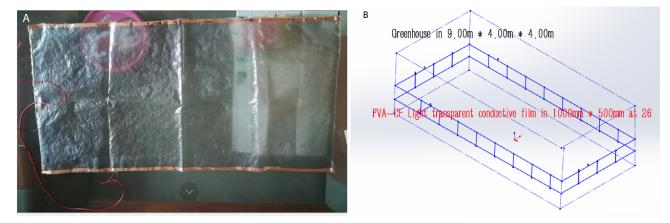
Figure 15: The PVA-CF Light Transparent conductive film be installed on greenhouse wall. (a) PVA-CF transparent conductive film. (b) Installation of 26 sheets of PVA-CF to the custom built agricultural greenhouse.
