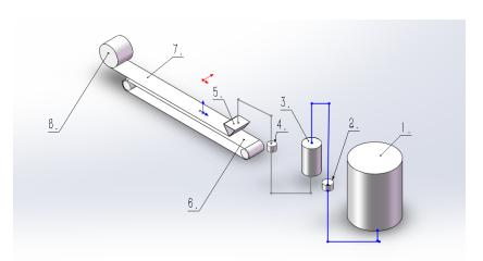
Figure 12: Fabrication machine for basic flexible conductive PVA-CF. 1: Mixer drum for mixing and blending of PVA, CF and glycerin. 2 & 4: pump. 3: Vacuum cavitation cylinder. 5: Horizontal slit funnel. 6: Heated conveyor steel belt. 7: PVA-CF film. 8: Winding machine.
