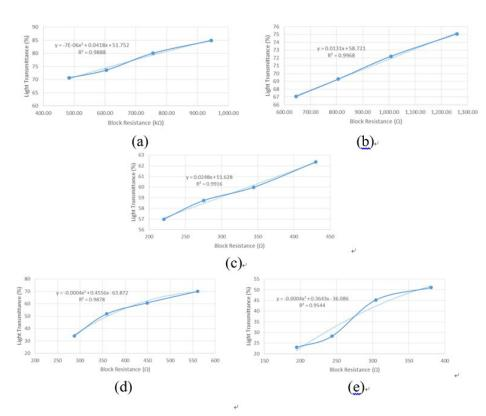
Figure 9: the relationship on the sample for Light Transmissivity vs. Block Resistance with Equations for CF-PVA. (a) Sample-01, CF:PVA of 0.1:30, (b) Sample-02, CF:PVA of 0.2:30, (c) Sample-03, CF:PVA of 0.3:30, (d) Sample-04, CF:PVA of 0.6:30, (e) Sample-05, CF:PVA of 1.0:30.
