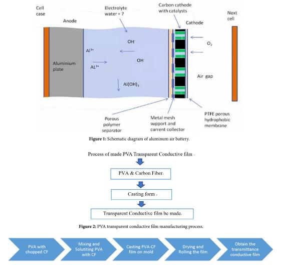
Figure 3: the process of fabricate polyvinyl alcohol with carbon fiber transmittance conductive film.
