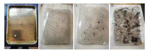
Figure 6: Casted film with carbon fiber in PVA solution: (a) Casting mold. (b) Film with 3mm CF filament. (b) Film with 6mm CF filament. (d) Film with 10mm CF filament.
