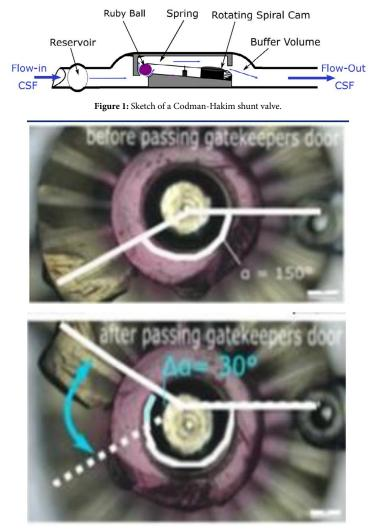
Figure 1: Sketch of a Codman-Hakim shunt valve.
